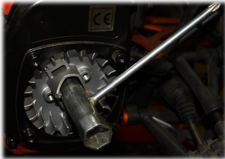
6. Install TR Dog Cage assembly (“see dog cage assembly instructions”) use thread lock on M5x12 FlatHead. Rotate “cutouts” on dog cage against “ears” on flywheel then tighten M5x12 FlatHead.
