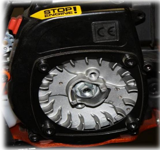
3. Remove Spark Plug and install piston stop.
