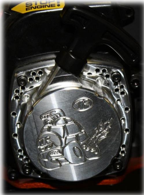
10. Rotate TR Housing assembly till the handle points in the direction you like and use 4pcs. M4x10SocketHeads to secure TR housing, holes in TR housing must line up with threaded holes in adapter plate. The holes in TR adapter plate are every 22.5degrees to offer you several options.
