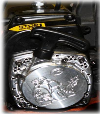
After install is finished, start the motor, if you here clicking noises at idle, turn your idle up till it stops.
