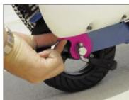
5) Lock Down quick release lever with snug pressure. This will lock axle in position until readjustment is required.
