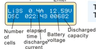
This shows the real-time status of discharging, you can press BATT TYPE/STOP key to stop discharging.
