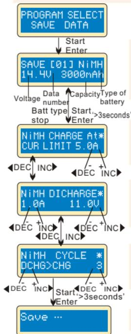
Setting of the parameter in the screen will not affect the charge and discharge process. They just present the specification of the battery. The example is NiMH battery pack, including 12 cells, the capacity is 3000m Ah.
