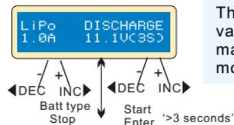
The value of discharge current on the left can not exceed 1C, and the value on the right can not be under the voltage recommended by the manufacturer to avoid deep discharging. Press START/ENTER for more than 3 seconds to start discharging.
