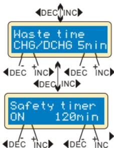
The battery becomes warm after cycles of charge/discharge process. The program will insert a time delay after each charge/discharge process to allow the battery enough time to cool down before beginning next cycle of charge/discharge process. The valid value ranges from 0 to 60 minutes.
