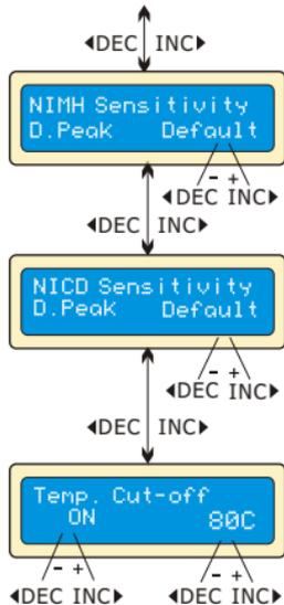
This shows the trigger voltage for automatic charge termination of NiMH and NiCd battery. The effective value ranges from 5 to 20mV per cell. If the trigger voltage is set higher, there is a danger of overcharging the battery; if it is set lower, there is a possibility of premature termination. Please refer the technical specification of the battery. (NiCd default: 12mV, NiMH default: 7mV)
