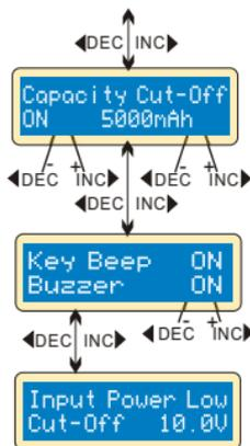
The program provides maximum capacity protection function. If the Delta-peak voltage can not be detected or the safety timer times out, the charge process will stop automatically, when the battery reaches the user-set maximum charge capacity,
